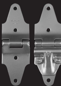
End hinge and roller carrier. Removable cap allows roller change without removing hinge.
